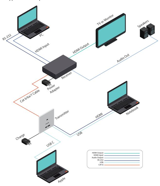
**EGE-6UHDC2-KVM-WTRL** 18Gbps HDBaseT 70M with USB-C/HDMI & KVM Function Wall Plate Transmitter
